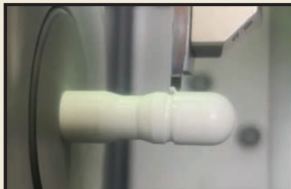
Micro-Line 1mm rad. Cutting Zirconium Oxide
